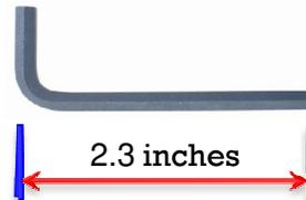
Torque = force times lever arm. Therefore to achieve 25 inch-lb force at a lever arm of 2.3 in., you only need to apply 11 lb force (near the weight of a 12 pack of soda)
