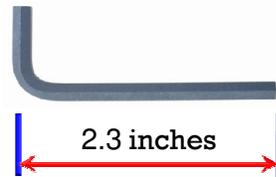
Torque = force \* lever arm. Therefore to achieve 25 inch-lb force at a lever arm of 2.3 in., you only need to apply 11 lb force (near the weight of a 12 pack of soda)
