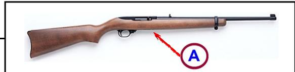
**Step 2** Replace with the Raven Eye Custom takedown screw. If you have a torque wrench, set it to 25 inch-lb MAX. If you are using the supplied wrench, read the HEX WRENCH NOTES section below.
