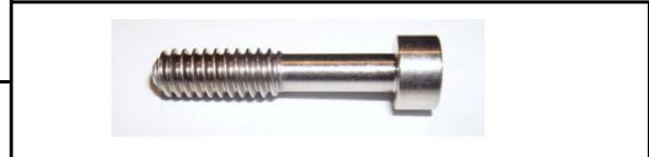
**HEX WRENCH NOTES** The 1/8" hex wrench is designed for a low torque application such as this. The goal is around 25 inch-lb torque. Of note is that most automotive tools measure in foot-lb, and do not go down to the 2 foot pound (25 inch-lb) range. If you are using the hex wrench and causing the wrench to bend, you are exceeding the 25 in-lb recommended. You may also damage the aluminum 10/22 action. The goal is repeatable torque not high torque. THIS ISN'T A STRONGMAN COMPETITION!
