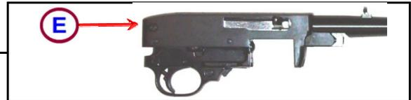
**Step 4** Replace with the new bolt buffer (F) in the same location. A small amount of gun oil may help with the insertion of the buffer.
